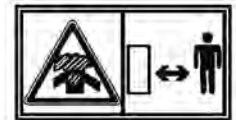
The exhaust gases are dangerous. Do not use in a poor ventilated area.
